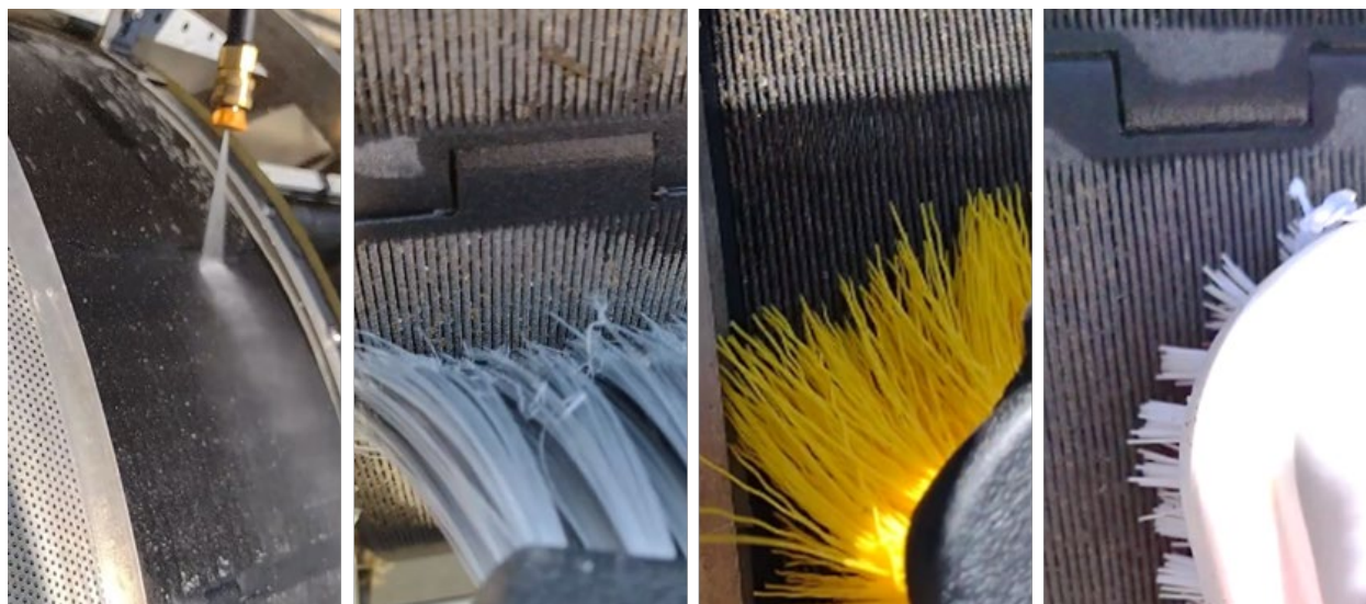
Figure 7 | Screen cleaning methods , left to right: water jetting, soft brush #1, medium brush #2, and hard brush #3.
